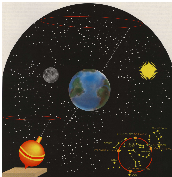
Figure 2: Precession of the equinoxes. The Earth is not perfectly spherical, but slightly oblate, with flattened poles and an equatorial bulge. Under the gravitational action of the Sun and Moon, its axis of rotation traces out a cone, much like a spinning top. The Earth's rotation axis traces out a large circle in the celestial sphere approximately once every 26,000 years. 5000 years ago the North Pole was indicated by the star Alpha, in Draco, rather than by Polaris. In 13,000 years, this direction will be indicated by Vega.
